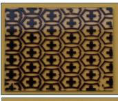
Two-layer structuring with SX AR-PC 5000/41 and AR-P 3250 (on the left resist mask, on the right after etching in glass)
