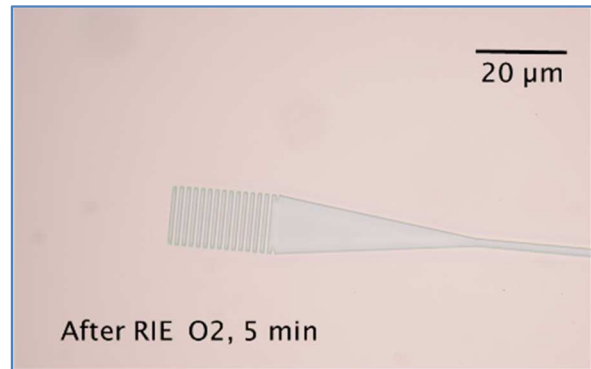
Fig. 10 Medusa structures after \text{O}_2 etching, film thickness still 140 nm
