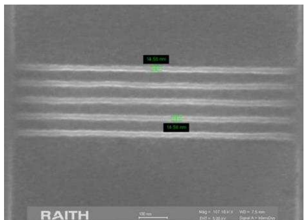
Fig. 4 14-nm lines produced with Medusa 82 SX AR-N 8200.03/2 (with PAG), dosage 1290 \mu\text{C}/\text{cm}^2
