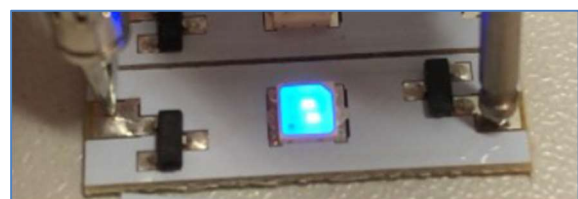
Fig. 2 Blue LED without casting compound with quantum dots
