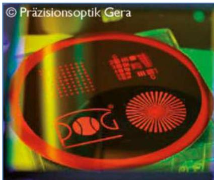
Fig. 13 Fluorescent PMMA structures after by e-beam exposure
