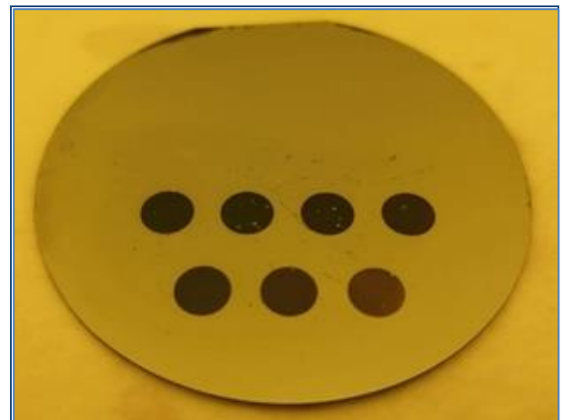
Fig. 7 Gradation curve (photolithography) with Medusa
