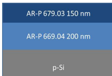
Layer structure of the two-layer system 600K/950K
