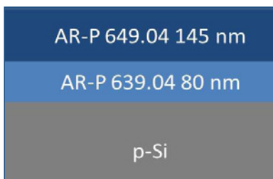
Layer structure of the two-layer system 50K/200K
