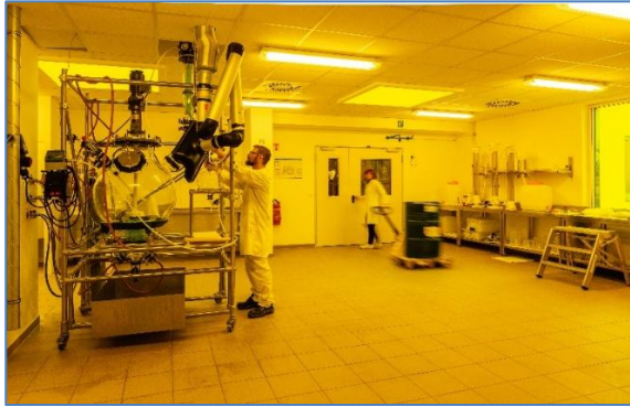
Fig. 6 Allresist production facilities with 200-litre-synthesis reactor "Frida"
