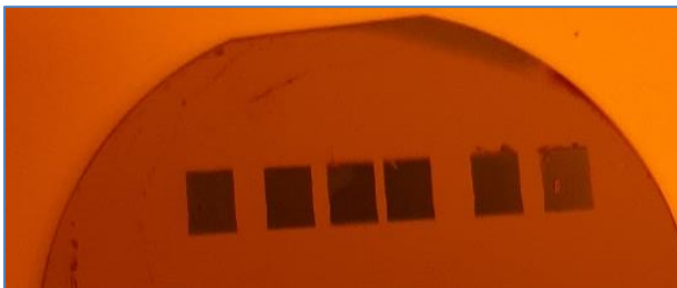
Fig. 4 Example of structured AR-PC 5090.02 (black squares, conductivity: 0.05 S/cm, developed with AR-N 4340 in a two-layer process) on a silicon wafer
