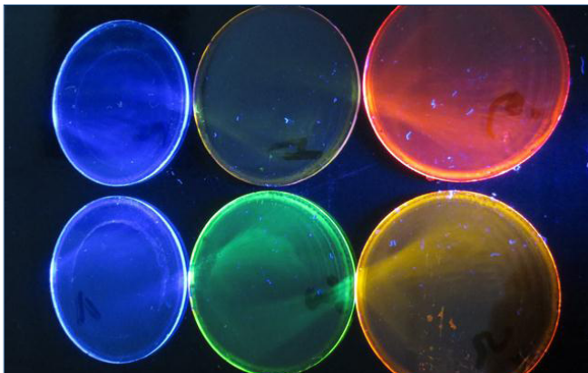
Differently fluorescing Atlas 46 films (irradiation with black light)
