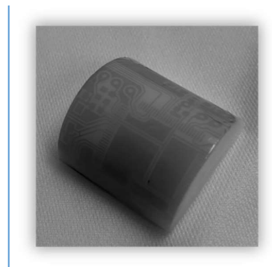
Fig. 7 The substrate after exposure and development
