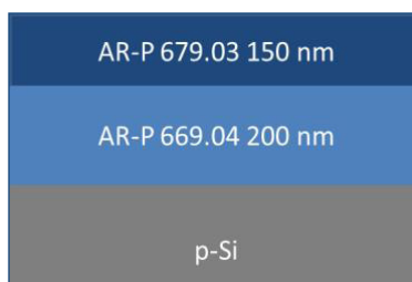
Layer structure of the two-layer system 600K/950K
